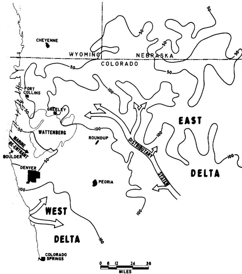
FIG. 3—Delta-sand isolith, "J" sandstone, Denver basin (modified from Haun, 1963).
