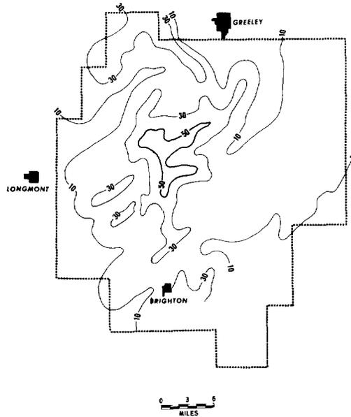
FIG. 6—Wattenberg field, net-"pay" isopach map, based on log calculations; 8 percent or more porosity, 60 percent or less water saturation. Contours are in feet.
