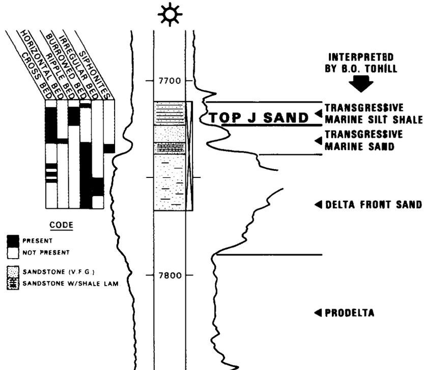
FIG. 9—Environmental interpretation of electric log and core data (Tohill, 1972).
