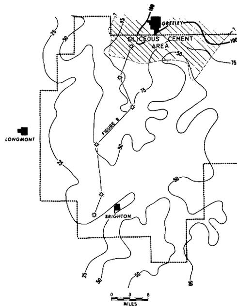
FIG. 7—"J" sandstone isolith, Wattenberg field. C. I. = 25 ft. Location of cross section (Fig. 8) is shown.
